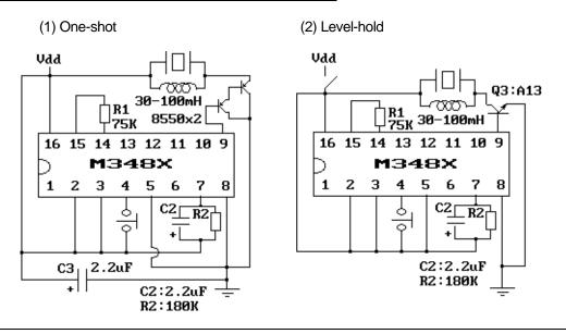
The inductor in parallel can be replaced by a  $100k\Omega$  resistor but the sound level will be lower.
